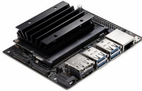
Figure 5 - Jetson Nano Developer Kit [12]
